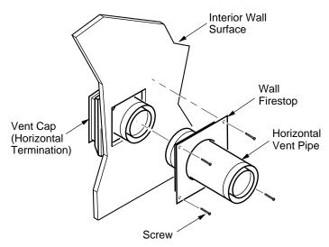
Figure 12 - Connecting Vent Cap with Horizontal Vent Pipe
